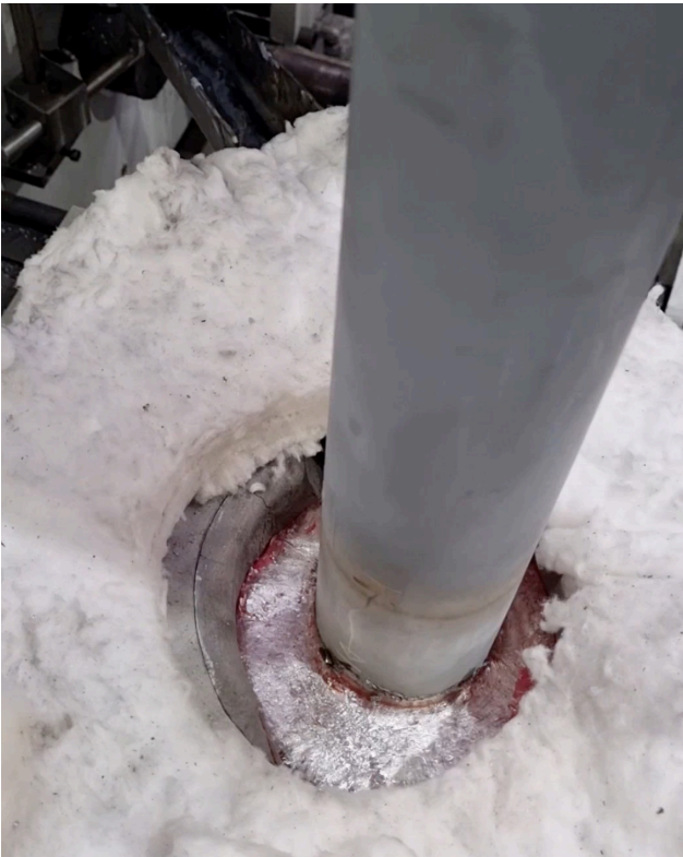
Fig. 6 Sonotrode submerged in US metal treatment unit
