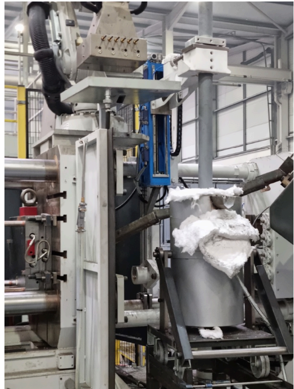
Fig. 7 - Industrial set-up MMM-Ultrasonic Treatment in Foundry
